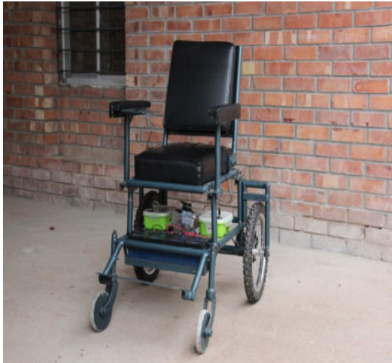
Fig. 8: Android controlled smart wheelchair for disabilities.
